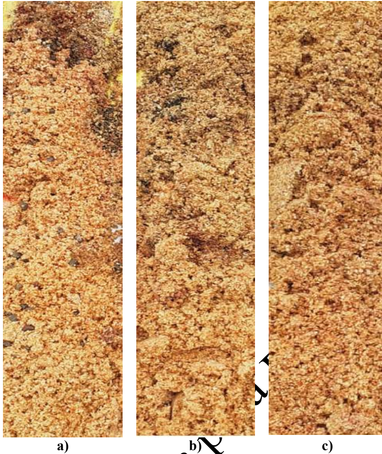
Figure 53. a) Control: MPF feed with drinking water b) MPF at the saturation with triclosan c) MPF duplicated. HRL=2 m 3 /m 2 -d.
